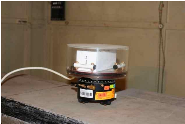
Figure 1. XYZ ring-core type Fluxgate sensor of the magnetometer installed at the Huancayo Observatory by the GRL, Tokyo University.
