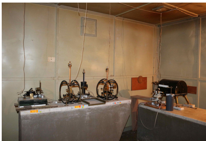
Figure 2. DTM Eschenhagen variometer and the digital system constructed by Erick Vidal at the Huancayo Observatory.
