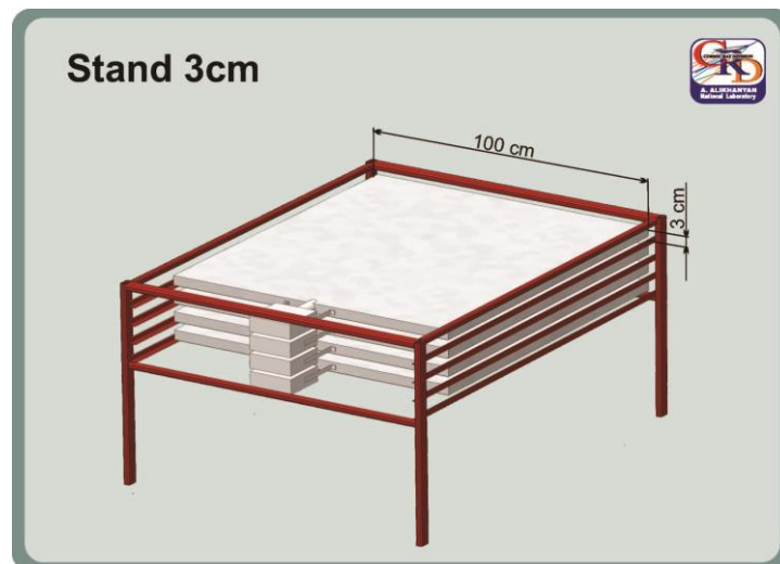
Figure 1. STAN3 detector measuring charged and neutral species of secondary cosmic rays
