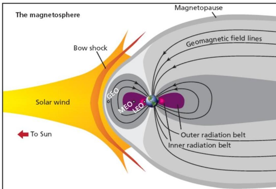
Figure 2. Schematic of the Earth's magnetosphere, with several regions labeled where satellite anomalies often occur, including the Van Allen Radiation Belts (Inner and Outer), and typical satellite orbits (GEO, MEO, and LEO). Courtesy of RAND Corporation, [www.RAND.org](http://www.RAND.org)
