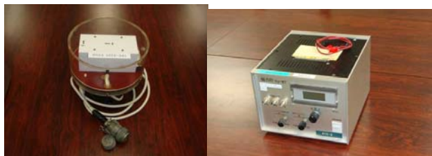
Fig. 3. YU-8T analog magnetometer (3-component magnetic field sensor at left and its analog amplifier at right)
