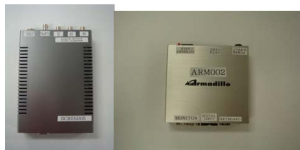
Fig. 4. Digital portion of MAGDAS-II system (DCR5SD analog-to-digital converter at left and Armadillo 9 Linux computer at right)
