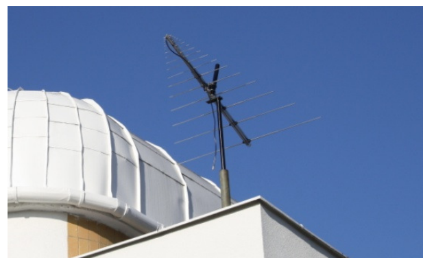
Figure 2: A log-periodic antenna CLP-5130-2N for the CALLISTO in Hurbanovo.
