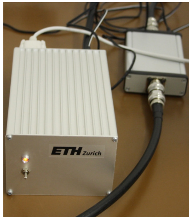
Figure 1: CALLISTO instrument No. eC50 (left) with the amplifier ZX60-33LN+.
