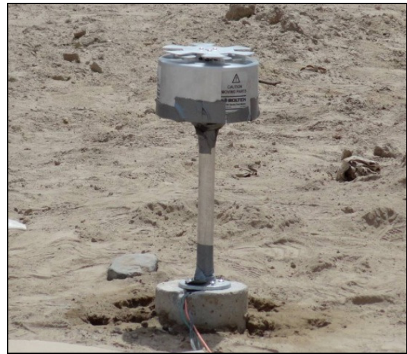
Figure 3: Final position of the EFM sensor installed at ICA University.
